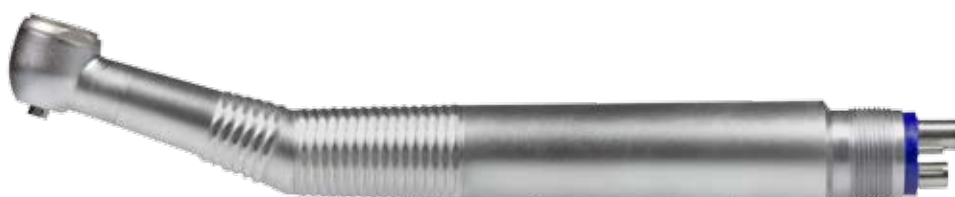
HC2012 - Power head, 1-port spray, ceramic-bearings, comfort-pushbutton-system, 18 Watt power at 340.000 rpm, fits for 4-hole tubings
